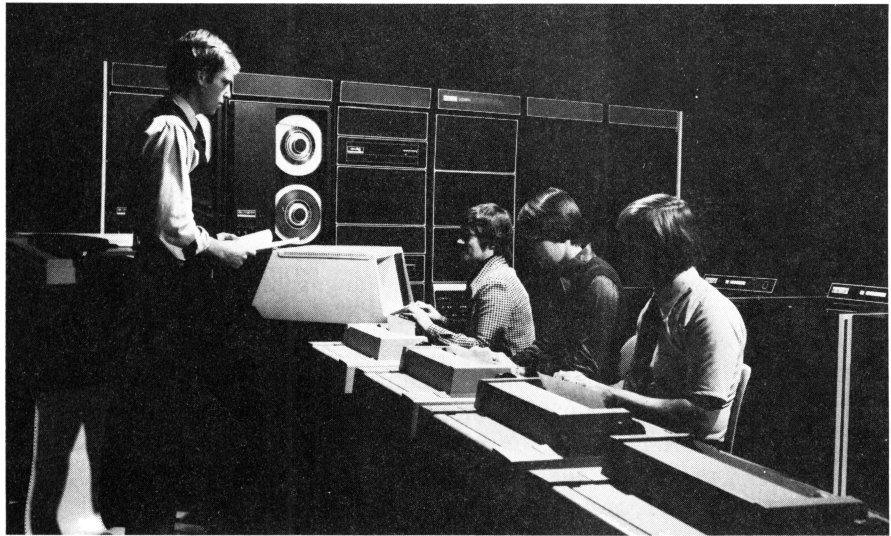
Figure 1.4 PDP-11/70 Computer System (Courtesy of Digital Equipment Corp.)
